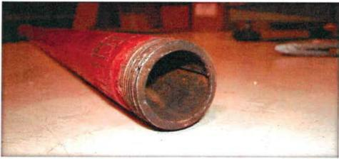
THIS IS NOT JUST THEORY; USING 99% NITROGEN INERTING REALLY DOES SOLVE THE CORROSION PROBLEM IN THESE SYSTEMS!
